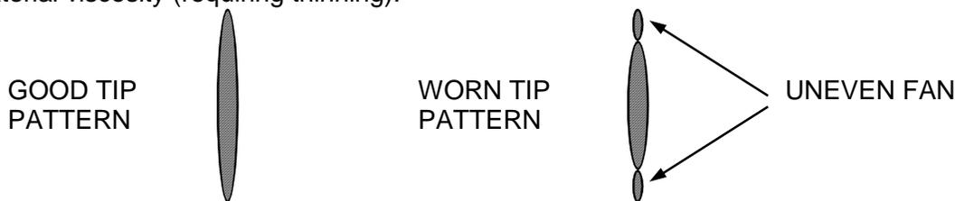
**NOTE:** Use of excessively worn tip can result in apparent poor performance of pump.
