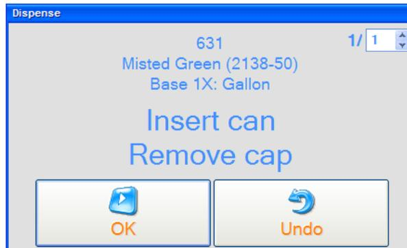
After selecting DISPENSE the above window will appear. This is a safety feature to insure there is a can under the nozzle and that the cap covering the nozzles has moved out of the way. If the correct can size is under the nozzles and the cap is out of the way then select OK to dispense.
