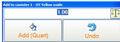
The colorant levels can also be changed by clicking on the field showing the numerical quantity of colorant (to the left of the fill canister icon) on the canister screen, typing the appropriate amount and pressing enter. The colorant bar will change automatically.
